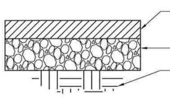
3" MIN. ASPHALT CONCRETE CL 1/2" PG 64-22 SEE SECTION 600 FOR ASPHALT CONCRETE SPECIFICATIONS
